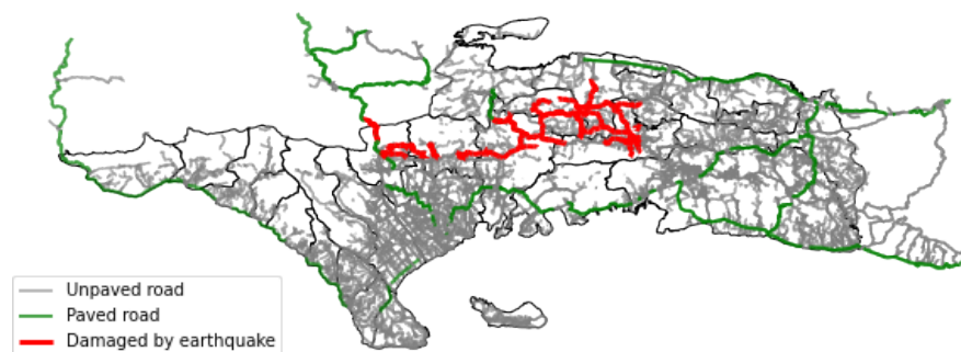
Figure 1: Road network of Sud and Nippes, including roads assessed as damaged by the August 2021 earthquake
