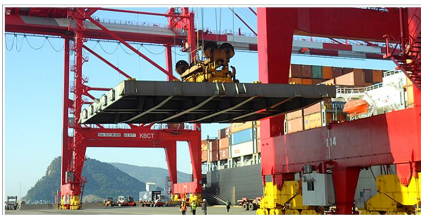
Figure 3. Vessel to Berth Hatch Move
