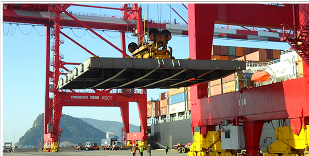
Figure 5. Ship-to-Shore Hatch Cover Move
