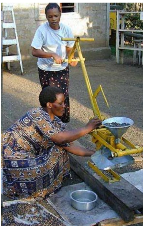
Figure 24. Bielenberg Hand Ram Press, Tanzania
