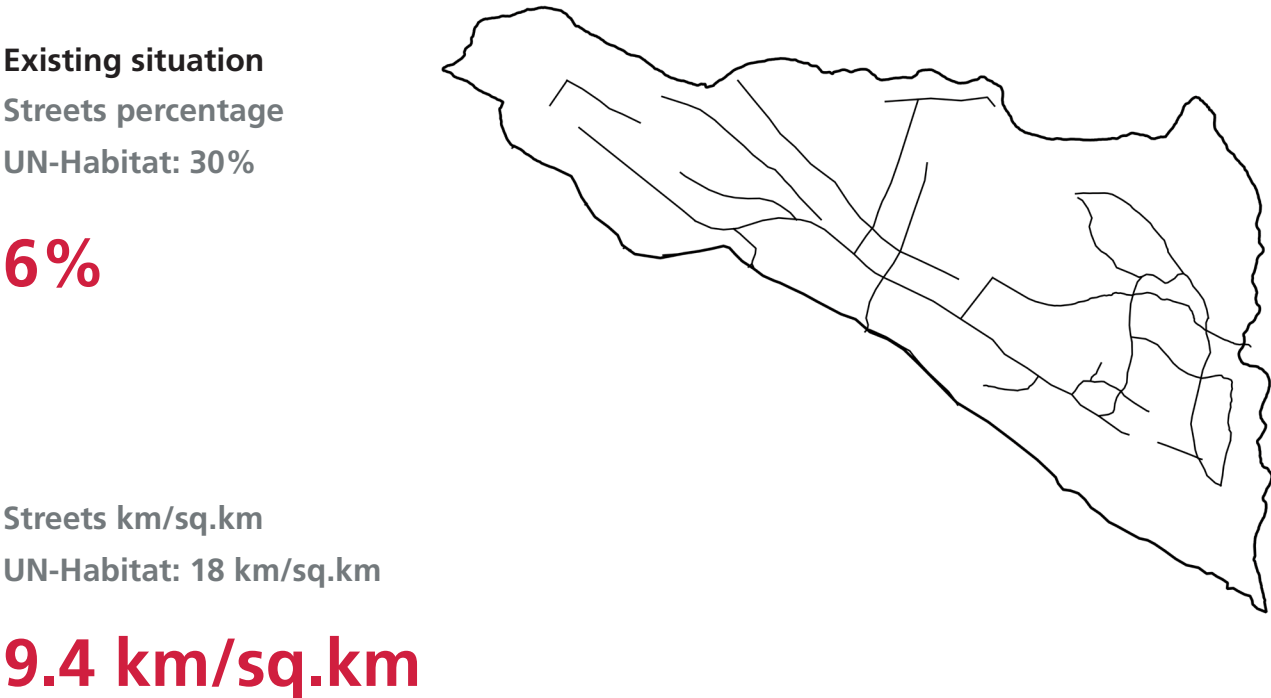
Fig. 165: Sources puantes: existing street network
