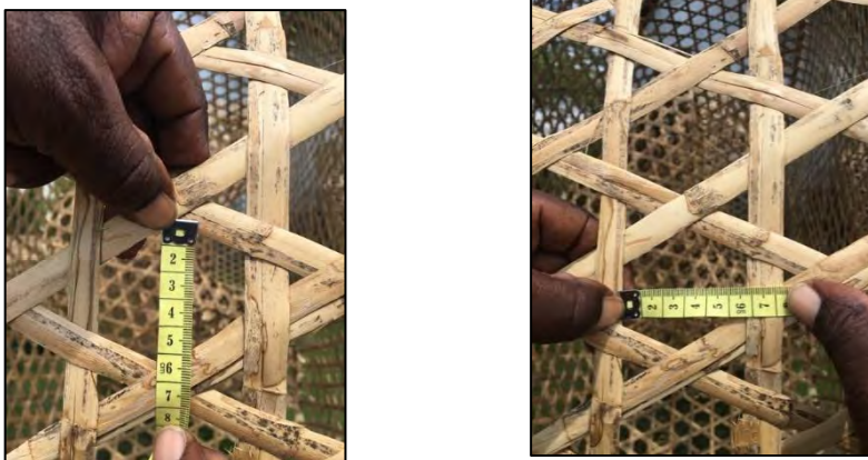
Figure 2. GPSS trap mesh with increased gap size of 6.5 cm x 6.5 cm.
