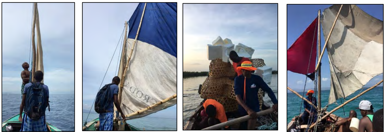
Figure 7. Fishers use wooden pirogues, bamboo oars and masts with sails sown together from pieces of material.
