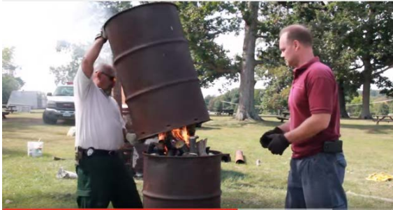
Putting after-burner chimney on barrel of burning wood soon to be charcoal
