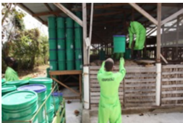
Figure 21. SOIL composting site. Transfer of container content to composting bins and disinfection of cleaned buckets with chlorine solution. Photo credit: SOIL (left) and Lars Schoebitz (right)
