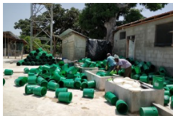
Figure 21. SOIL composting site. Transfer of container content to composting bins and disinfection of cleaned buckets with chlorine solution. Photo credit: SOIL (left) and Lars Schoebitz (right)
