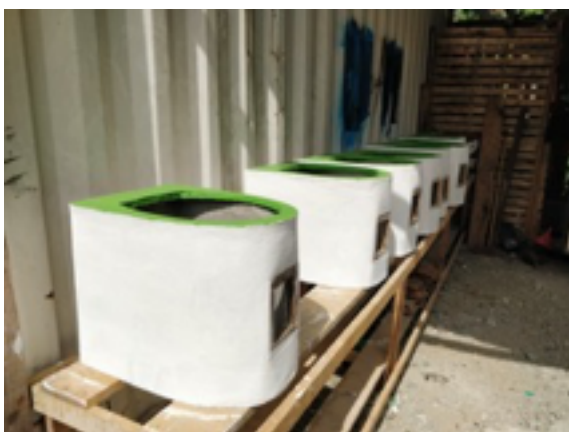
Figure 13. Construction of SOIL CBS toilets using locally available materials (concrete). Photo credit: SOIL
