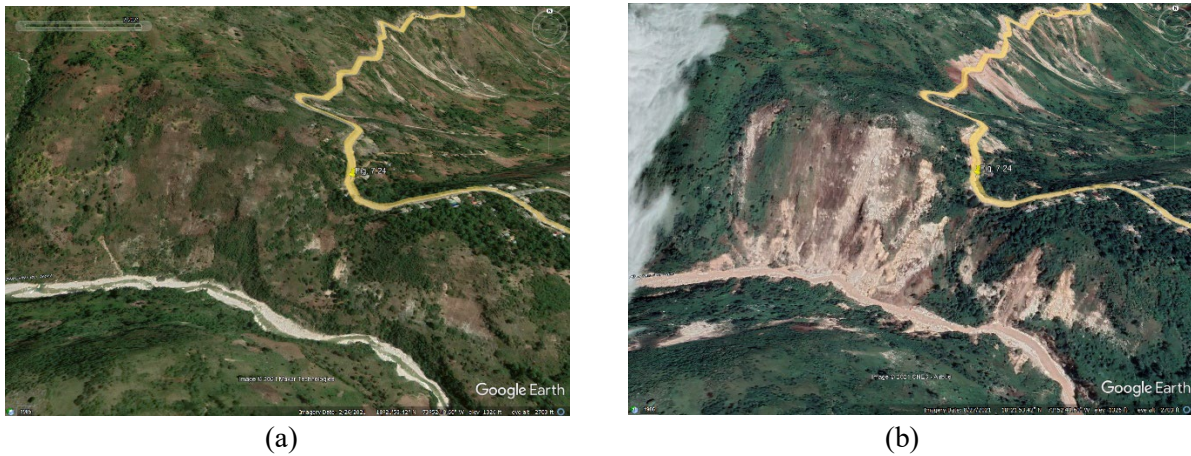
Figure 7.27. Pre-event and post-event satellite imagery of landsliding along RN7 west of Champlois (courtesy of Planet Labs, planet.com): (a) February 26, 2021. (b) August 27, 2021.
