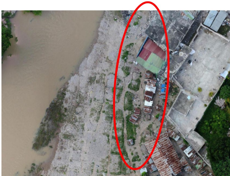
Figure 7.97. Damage and possible lateral spreading near river (Riviere de Cavaillon) in Cavaillon. Coordinates: 18.299167, -73.655833. Images courtesy of OpenstreetMap (Pierre Béland, https://pierzen.dev.openstreetmap.org/ ).
