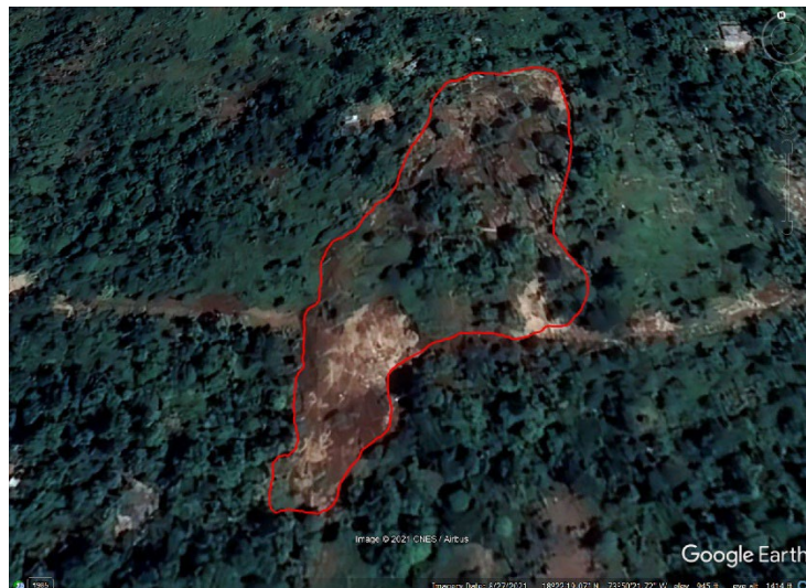
Figure 7.23. Satellite imagery of Landslide (roughly outlined in red) shown in Fig. 7.22 (courtesy of Google Earth).
