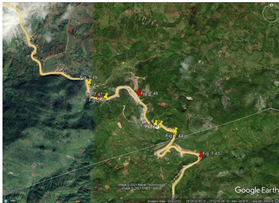
Figure 7.42. Locations of landslides (yellow pins) and rockfalls (red pins) observed along RN7 (courtesy of Google Earth). Imagery date October 9, 2021.
