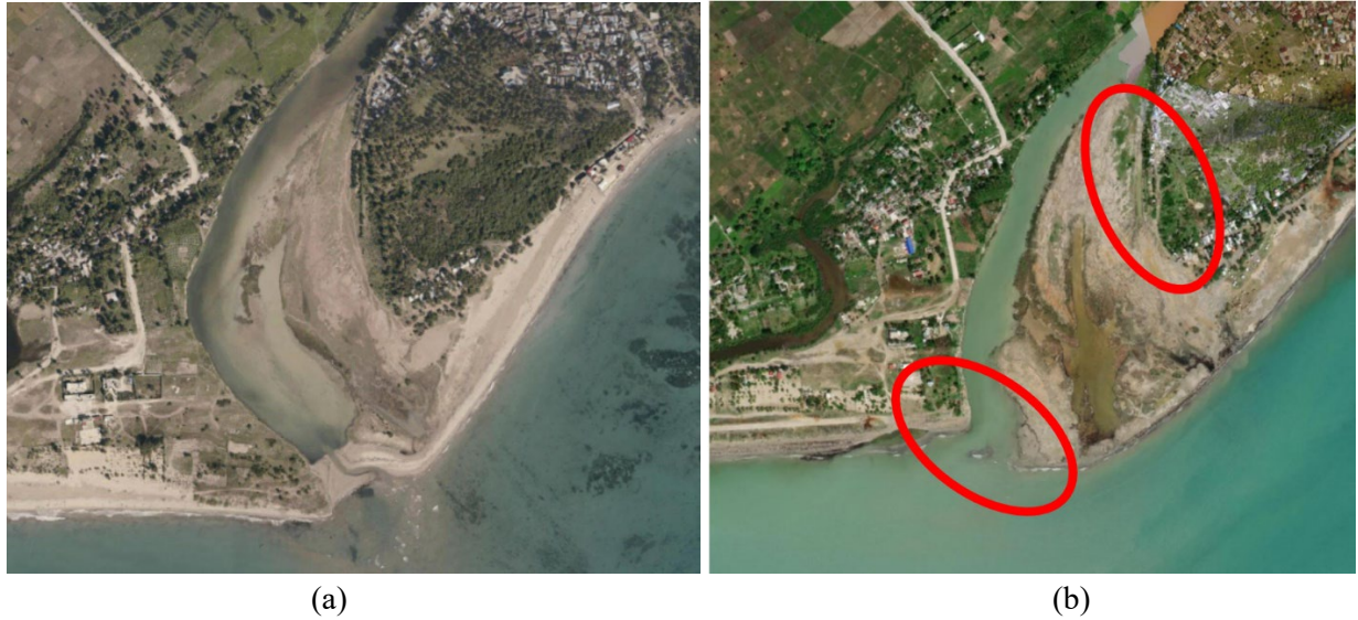
Figure 7.87. Coast and slope damage near south Les Cayes: (a) before the earthquake; (b) after the earthquake. Coordinates: 18.181111, -73.758611. Images courtesy of OpenstreetMap (Pierre Béland, https://pierzen.dev.openstreetmap.org/ ).
